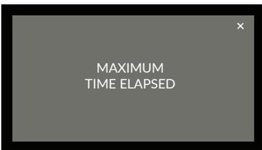
After 48 h the appliance finishes the cycle in progress and emits three sound signals. The display shows the message "maximum time elapsed". By pressing
