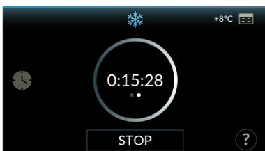
Press on the central active area to view the time elapsed from the start of the blast chilling cycle with core probe.
