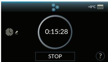
If freezing phase is in progress, by setting the time to zero you will switch to storage phase. The temperature inside the chamber detected by the air probe is shown at the top right-hand side.
