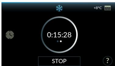
If cold maintenance is selected, after 10 seconds FREDDY sets automatically to blast chilling cycle, the displays shows the relevant cycle screen, in manual mode with timer and default values (2 h).
