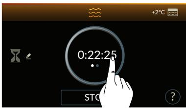
Press on the central active area to view the temperature set at the core of the food.
