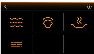
By pressing the hot functions key the screen shown on the side will be displayed. Press the
