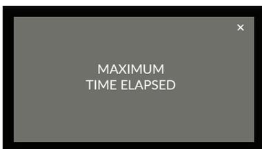
After 48 h the appliance finishes the cycle in progress and emits three sound signals. The display shows the message "maximum time elapsed".
