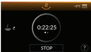
If the initial cold storage is not present (set time equal to zero) or is finished, the unit switches to reviving phase.
