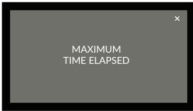
After 48 h the appliance finishes the cycle in progress and emits three sound signals. The display shows the message "maximum time elapsed". By pressing **X** in the "maximum time elapsed" information window you will go back to the main screen.
