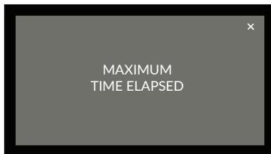
After 48 h the appliance finishes the cycle in progress and emits three sound signals. The display shows the message "maximum time elapsed". By pressing
