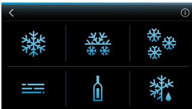
After 5 seconds of inactivity the names of the cycles relevant to the functions start to be slowly displayed in sequence. For the cold functions the order is the following: BLAST CHILLING +3 °C, SOFT FREEZING -18 °C, FREEZING -18 °C, MAINTENANCE, DRINKS CHILLING, DEFROSTING. For the hot functions the order is the following: LOW TEMPERATURE COOKING, RISING, READY MEAL, MAINTENANCE.
