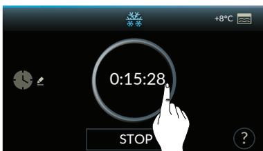
Press on the central active area to view the time elapsed from the start of the soft freezing cycle with core probe.
