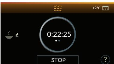
If the initial cold storage is not present (set time equal to zero) or is finished, the unit switches to low temperature cooking phase. The display shows the time left (countdown) of the low temperature cooking phase.
