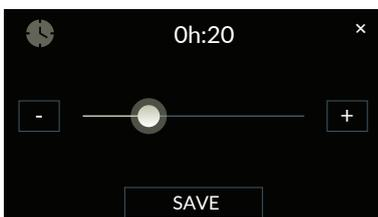
The screen for cleaning time setting will appear. (cleaning time can be set from 20 min. to 60 min.).
