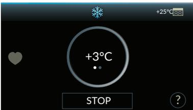
If cold maintenance is selected, after 10 seconds FREDDY sets automatically to blast chilling cycle, the displays shows the relevant cycle screen, in automatic mode with probe and default values (+3 °C). Cold maintenance, after blast chilling phase, can last up to 48 h.
