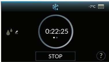
If the initial cold storage is not present (set time equal to zero) or is finished, the unit switches to defrosting phase.
