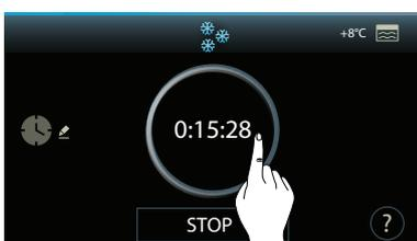
Press on the central active area to view the time elapsed from the start of the freezing cycle with core probe.
