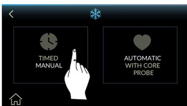
press "MANUAL WITH TIMER" and touch the central active icon ⌚ highlighted by the cycle time.
