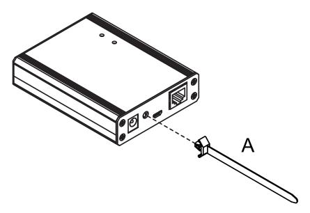
3. Insert the other end of the DC jack lock component A through the component B's joint.
