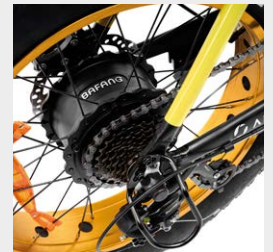
36V 250W 60Nm rear Bafang motor
