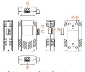
①RJ45 interface ②LED ③Switching amount ④Dial switch ⑤Wall mounting hole ⑥Magnets
