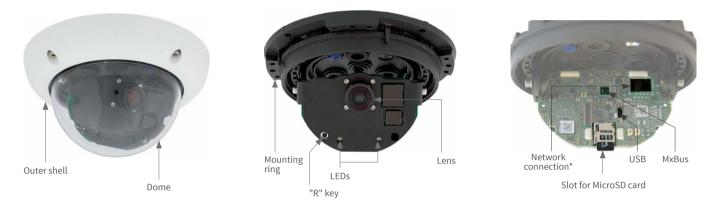
\*To suppress electromagnetic interference, attach the enclosed hinged ferrite (item 1.6) to the pre-installed Ethernet cable of the camera. The hinged ferrite should be positioned as close as possible to the camera body.
