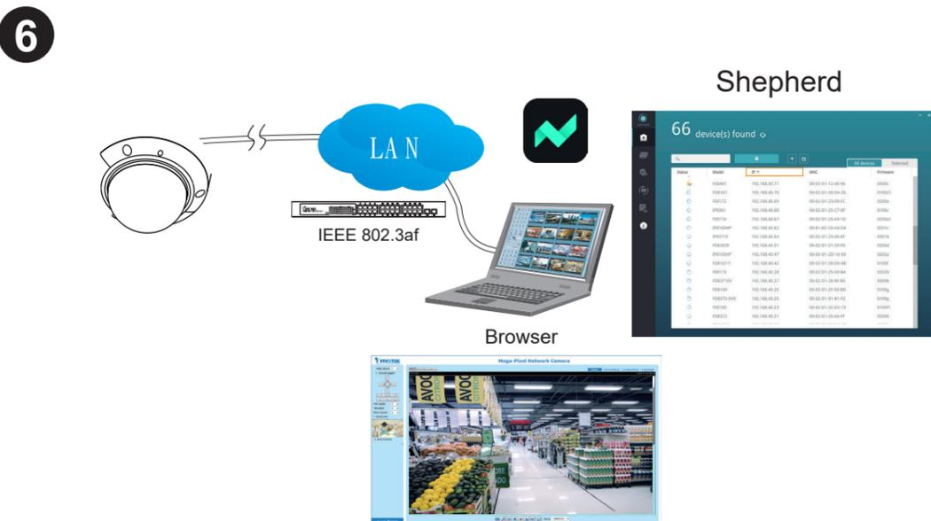
1. After connecting the network camera to the PoE network switch, run the VIVOTEK Shepherd app to search for the IP location of the network camera. Then, enter the camera's webpage.
