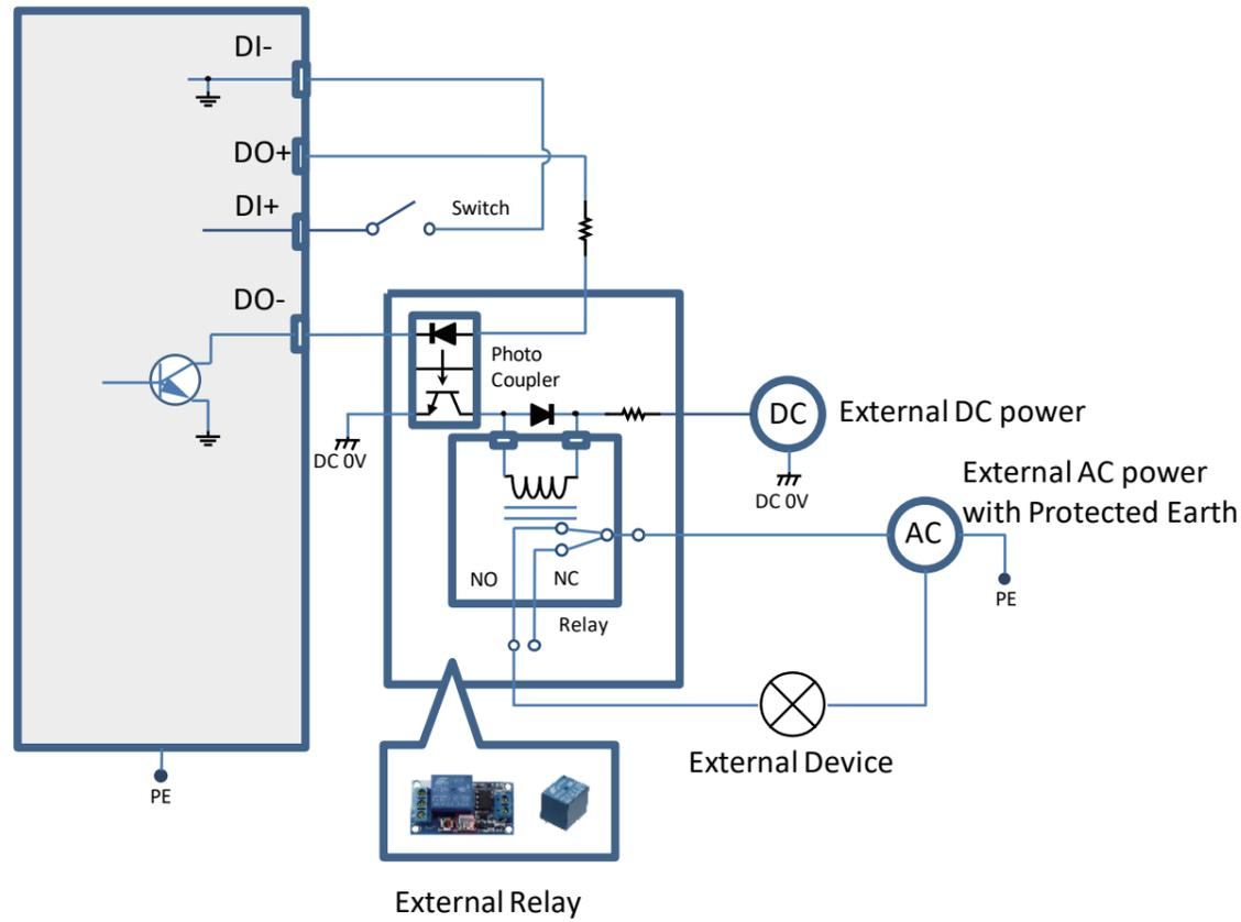
1. The DO+ pin provides 12V output voltage, and the max. load is 50mA.
